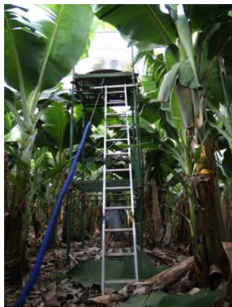
Class A evaporation pan installed at canopy level (about 4.5 m) in a screen house
