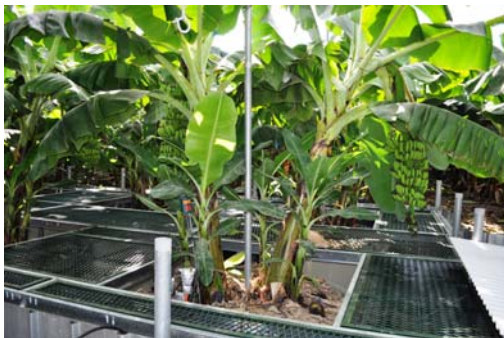
A steel floor is installed to facilitate horticultural work. It is not touching the lysimeters themselves.
